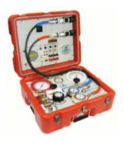
Kirby Morgan Air Control System 5 (KMACS 5) is a lightweight, portable control box for two diver use in surface supplied air diving operations. The KMACS 5 controls the diver's air supply, communications and monitors the diver's depth. It allows two divers clear push-to-talk (two wire) or round robin (four wire) communications. The KMACS 5 is also available without communications.
